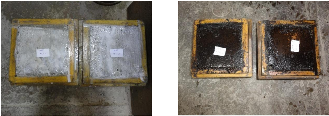
Figure 3. RCC specimens cured with different materials
