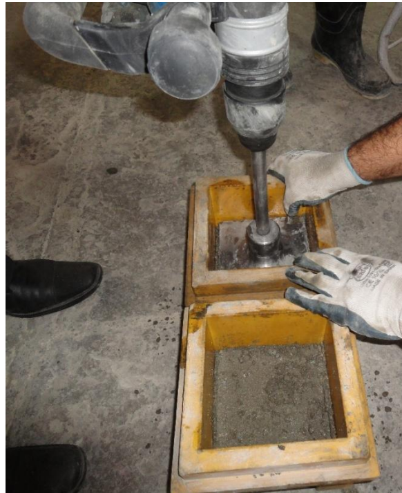
Figure 2. Molding and compaction of concrete specimens
